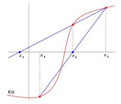
The first two iterations of the Newton's method for finding the root of the function f(x) The convergence behaviour of the sequence is the following:
