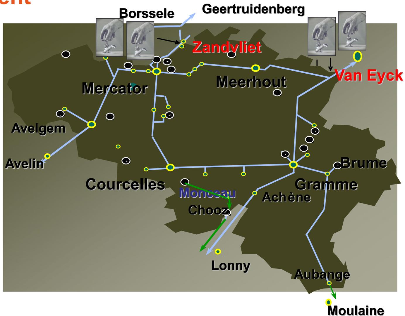
Installation of Phase Shifter Transformers on the Northern border for managing increasing Loop flows
