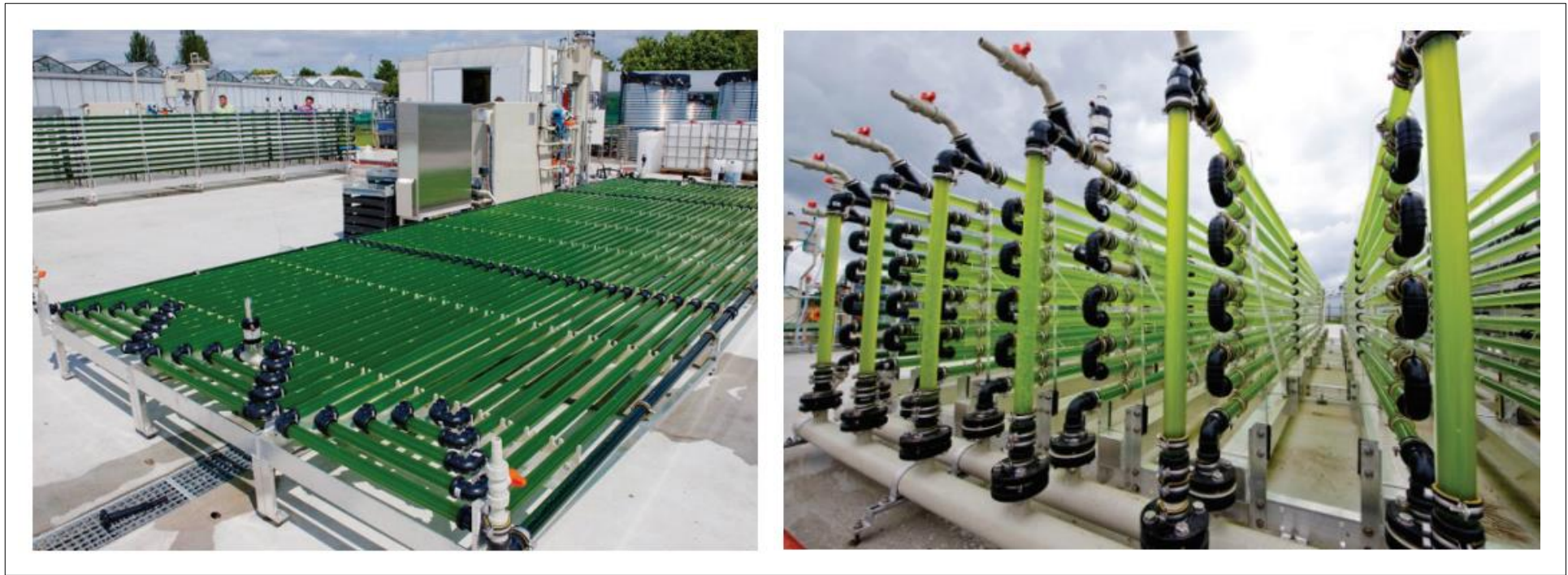
Figure 19: Horizontal and stacked tubular algae reactors consisting of several connected loops (Algae PARC Wageningen University).
